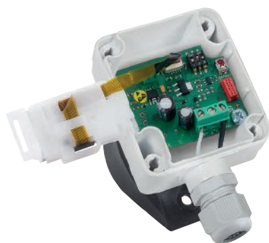
TM 65 with display and quick-locking screws (IP 65)
